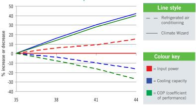
Outdoor Temperature (Degrees Celsius DB) Source: Uni SA Roxby Downs Report June 2009 Climate Wizard's cooling performance can rival that of refrigerated systems, using up to 80% less energy.
